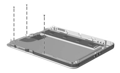
Removing the Bracket Screws
